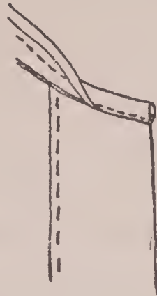
Fig. (13) The facing turned and stitched in its finished position
